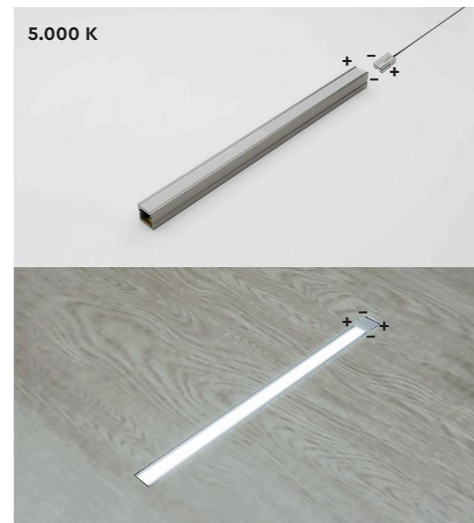
THE LIGHT TEMPERATURE CAN BE SET TO 2,700K OR 5,000K BY REVERSING THE CONNECTION DIRECTION OF THE FAST CONNECTOR.
